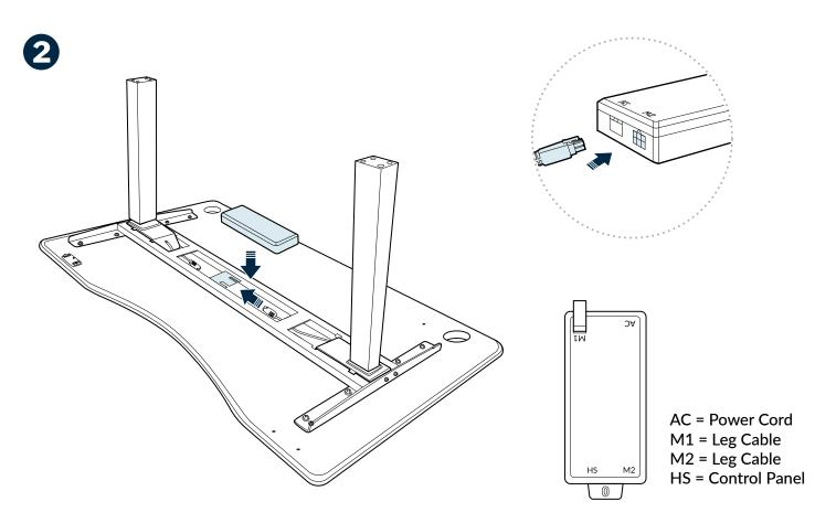
Once the legs are secured with screws and while the desk is still face down, lower the control box into the middle cavity of the metal frame. Then, slide the control box to engage the bracket that holds the control box in place. When the control box is secured, connect the leg cables to the corresponding control box inputs, M1 and M2.
