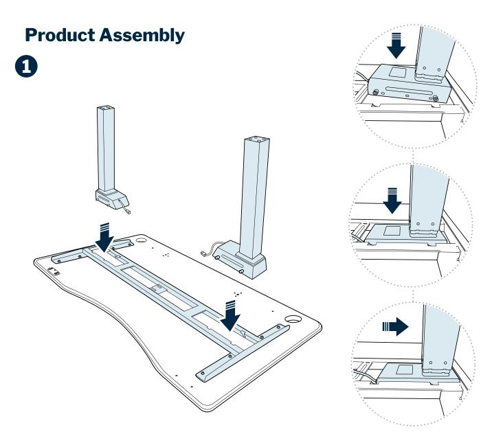
Desktop and desk legs will arrive in separate boxes. We recommend assembling the desk with the desktop face down in its box to prevent any surface scratching. Open both boxes; remove the desk legs and parts from their box.
